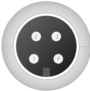
Figure 58.1. WH Control pinout diagram.
