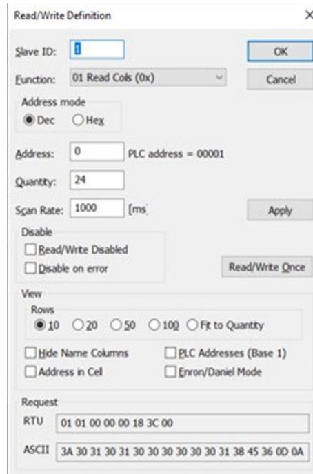
Figure 41.1. Read/Write Definition window.
