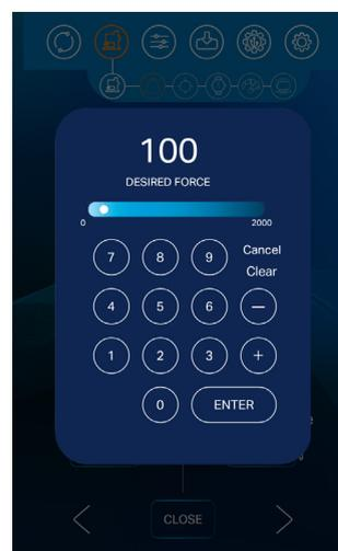
Figure 15.2. When you touch the Desired Force box a pop-up window will appear. You can use the slider bar or the number pad to enter the amount of force you desire, measured in grams.
