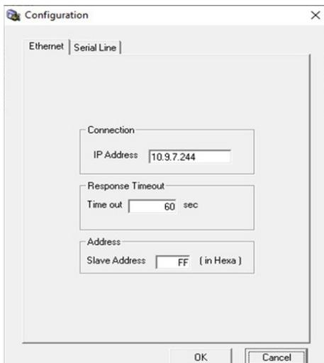
Figure 35.2. The Modbus Configuration screen.
