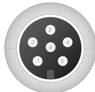
Figure 57.2. E-Stop pinout diagram.
