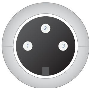
Figure 58.3. Secondary Trigger pinout diagram.
