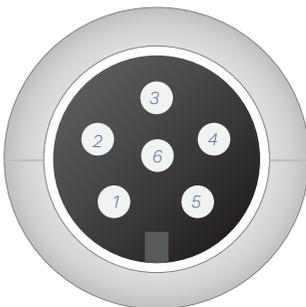
Figure 58.2. Primary Trigger pinout diagram.
